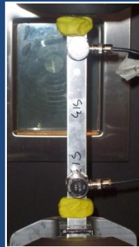
Notched Tensile Fatigue Specimen with Attached AE Transducers in MTS Machine
